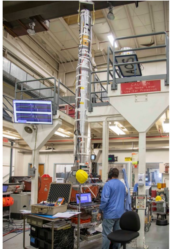
INFUSE payload vibration testing. Credit: Berit Bland/NSROC
